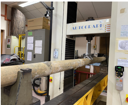
Figure 2. Arrangement for 3-point static bending test of 3-meter-long bamboo culms
